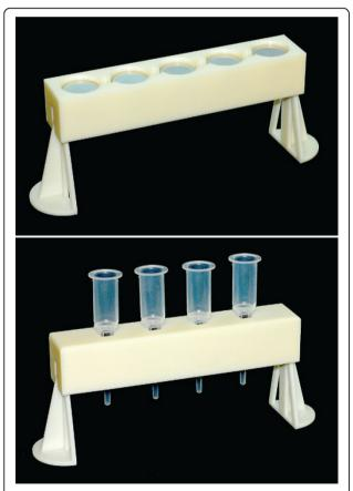
**Figure 3 Magnetic purification stand**. Photographs of the designed magnetic purification stand. (A) The stand with the lid removed showing the cylinder magnets. (B) The complete stand with four LS columns in place for purification. A disposable trough commonly used in high-throughput microplate applications fits beneath the column nozzles.
